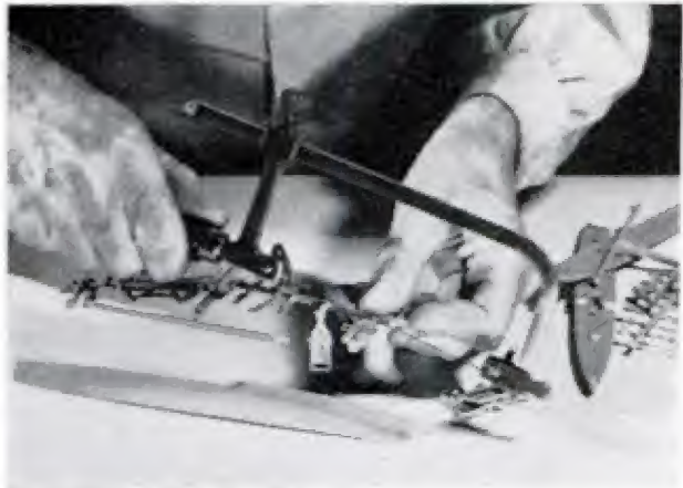
ON MODEL WORK , jeweler's blade produces extremely fine cut and seldom requires further finishing
